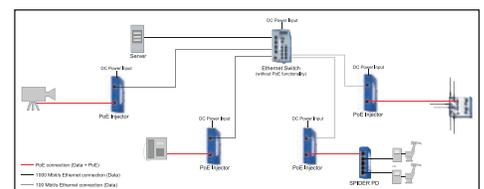
Example of PoE Injector Installation Illustrating the use of PoE.
