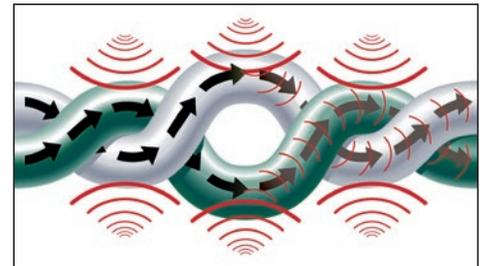
**Illustration 1:** Example of Non-Bonded-Pair. As cable is stretched and pulled, pairs begin to separate, causing a degradation in signal quality.
