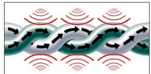
**Illustration 2:** Example of Bonded-Pair. As cable is stretched and pulled, pairs stay intact.
