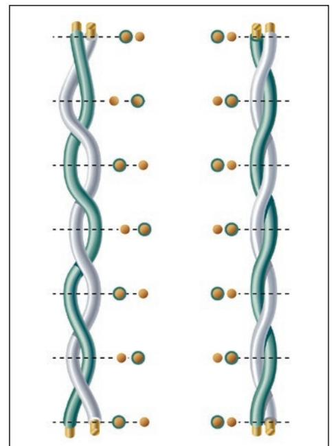
**Illustration 3:** Side-by-side comparison. Non-Bonded-Pair versus Bonded-Pair cable.
